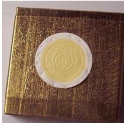
Figure 7.1: E. coli C bacteria were deposited on a membrane filter with 0.45 \mu\text{m} pore size. The filter was mounted on a brass sample which can be fitted easily inside the chamber. Details of the filter study are provided below.
